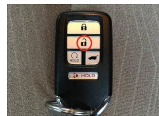
Control from key fob by pressing unlock button 4 times
